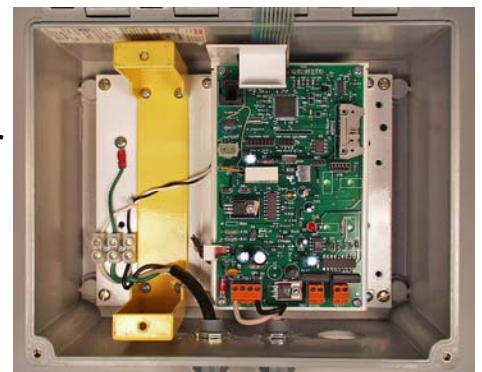
Control Box Inside
